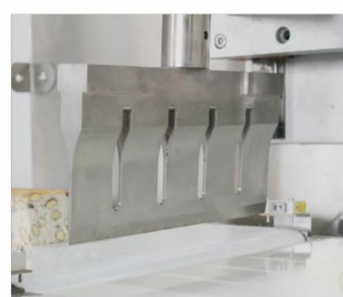
UFM3500 Automatic Ultrasonic Food Slicing Machine is a fully automatic high-performance food cutting equipment with multiaxis standard control system. It can be used for round portion mode and slice mode. Compared with ordinary cutting machines, it could be reduced the amount of food scrap, increased productivity, enhanced the food surface aesthetics greatly. It is a strong promoter to join the ultrasonic in the brand competition.
